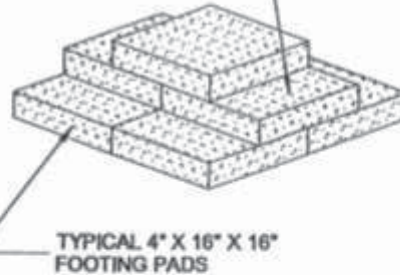
1024 SQ IN PIER PAD (11,000 POUND CAPACITY) FIGURE 403.5
